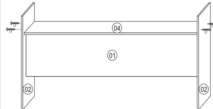
**4** \*\*\*Fixar o painel superior com parafusos e fixar as cantoneiras unindo o painel horizontal com o painel inferior
