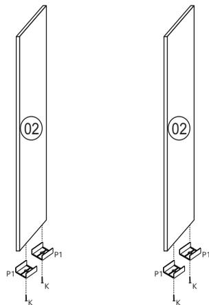
**2** \*\*\*Fixar as laterais no painel inferior com parafusos
